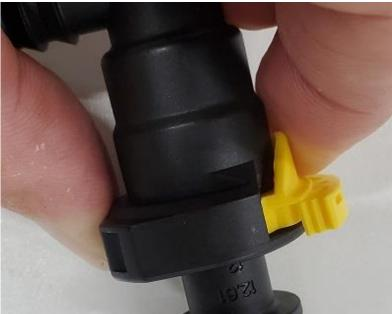
Tab Unlocked, Button pressed to release
